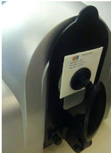
6. Select the button “Auto-Calibrator”. The instrument will measure the standard and try to position the filter wheel to adjust the UV content to the value of the standard +/- 1 CIE whiteness units.
